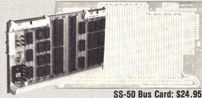
I/O card is 1-¼ inches higher than SWTP I/O card • interdigitated power conductors . contacts for power regulators and distributed capacitance bypassing use wire wrap, wiring pencil or solder wiring • tin-lead plating over 2-oz copper conductors wets quickly, solders easily FR4-G10 epoxy-glass substrate.
